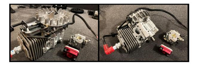
Install the Electric Starter Adapter.
