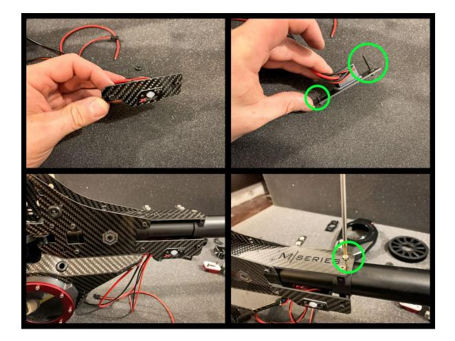
2<sup>nd</sup> Stage Gear Mesh Adjustment.
