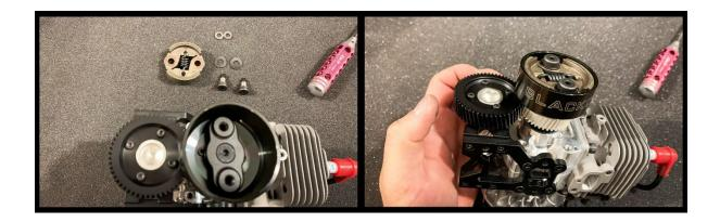
Engine/Gear Box Assembly Placement into Monocoque Frame.
